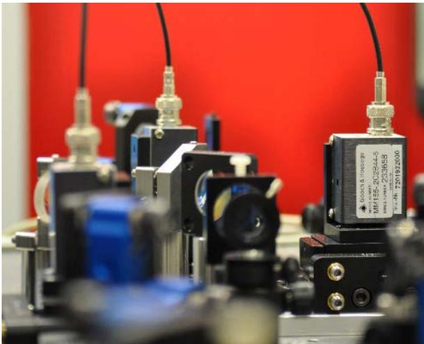
*Setup for phase-modulated interferometry*
