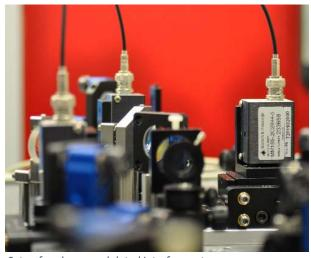
Setup for phase-modulated interferometry
