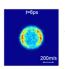
RbHe<sup>+</sup> Velocity-map ion images recorded at different pump-probe delays between excitation and ionization.
